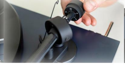
Balance the tonearm so it stays level by turning the counterweight forwards and backwards on the rod.
