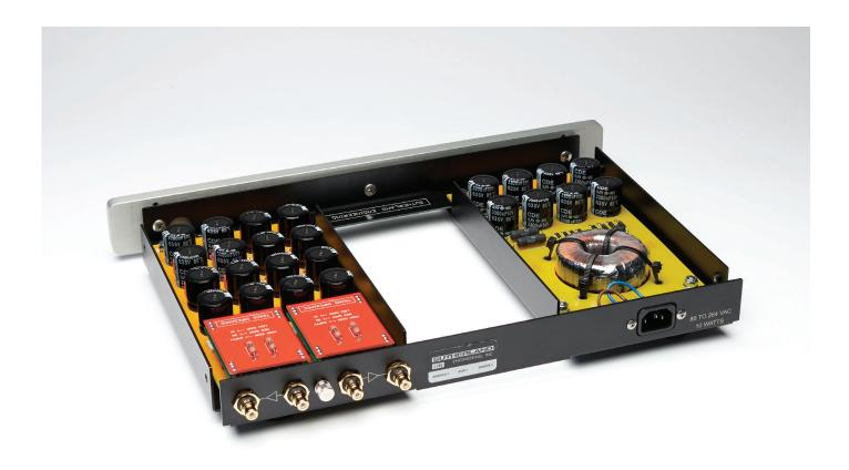
The connections on the back panel of the **little LOCO** appear totally conventional. There is the usual IEC input for the power cord, a ground screw for grounding the turntable, and two RCA jacks for the input signal from the turntable. Finally, two RCA jacks deliver an output signal to your line-level preamp.
