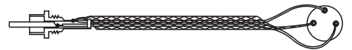
Detail of twin cored screened lead connecting phono to XLR plugs (pre-amp to x-over)
