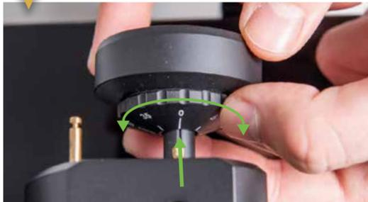
**18** Turn the WHOLE counterweight counterclockwise until the scale reads 23.
