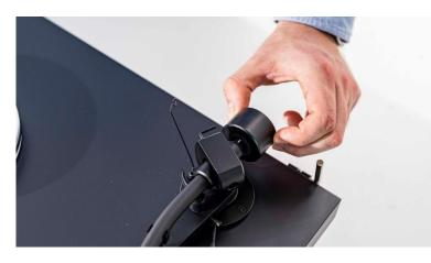
Pushing carefully, move the counterweight (6) onto the rear end of the counterweight support rod as shown in the picture below. Place the stylus pressure gauge onto the platter. To set the required VTF, lower the tonearm lift lever as indicated in the illustration and place the tip of the stylus exactly in the point marked 23mN (23mN = 2,3g). If the stylus gauge becomes level, then the correct pressure has been
