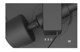
Slip the loop of the anti-skating weight's thread over the third groove of the stub to set the correct anti-skating force for the factory-fitted cartridge. Feed the thread through the loop of the wire support (17).
