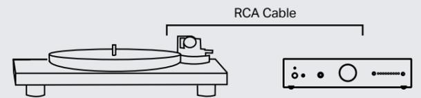
Deactivates the built in phono preamplifier in the A1. Connect to an amp with integrated MM phono input or use an external MM phono preamp.
