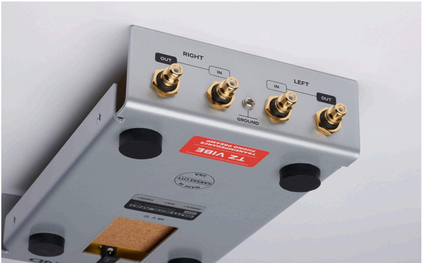
Place the **TZ VIBE** near the turntable. The turntable signal is applied to the two centrally located RCA jacks on the back panel. Often there is a ground wire coming from the turntable. Connect it to the grounding screw in the center of the back panel. The output of the **TZ VIBE** goes to a line-level input on your preamp or integrated amplifier.
