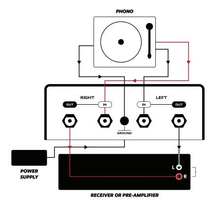
A basic turntable produces a low level signal. It must be amplified and equalized before going to a line level input (sometimes labeled AUX) of a preamplifier or receiver.
