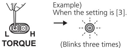
② To change the setting, press the H or L torque button while the lamp is lit two seconds.
