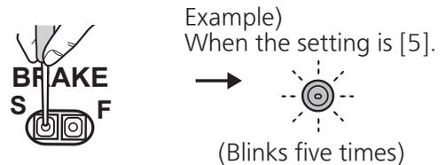
② To change the setting, press the F or S brake button while the lamp is lit two seconds.
