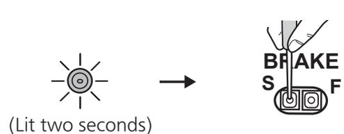
③ After you press the brake button, the confirmation lamp blinks the specified number of times showing the new setting, stays lit for two seconds and then goes off.
