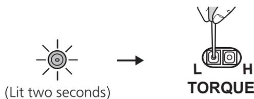
③ After you press the torque button, the confirmation lamp blinks the specified number of times showing the new setting, stays lit for two seconds and then goes off.
