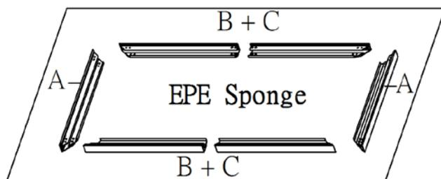
**Step 3.** Insert the center joint connectors into one-half of the horizontal frame and secure with the M4x6 screws (2 for both top and bottom). Once secure, connect the other half of the horizontal frame and fasten with the M4x6 screws (2 for both top and bottom).
