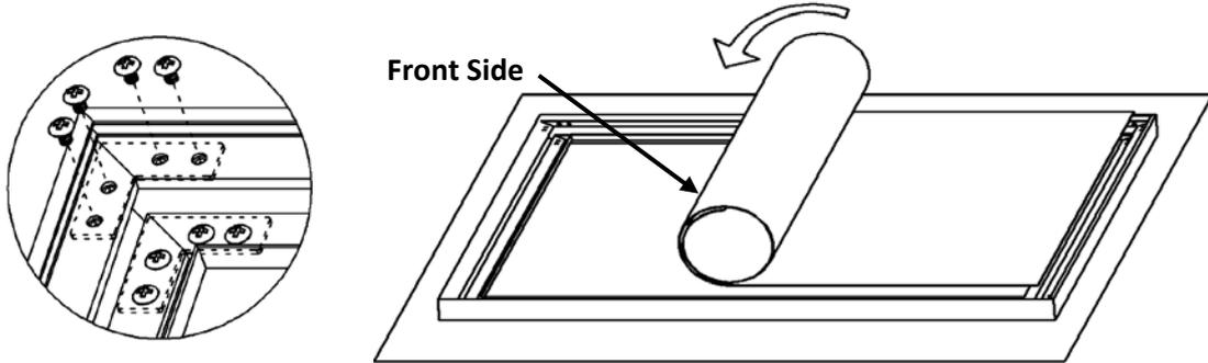
**Step 8.** With one end of the spring and secure inside the groove of the frame, hook the spring to the hole located on the screen material's outer edge. Use the pull hook when necessary. Attach the four corners first (1). After those are secure, connect the vertical portions of the material, begin in the center and move towards the corners (2). Lastly, connect the horizontal sections of the material by connecting the center of the material and make your way towards the corners (3).
