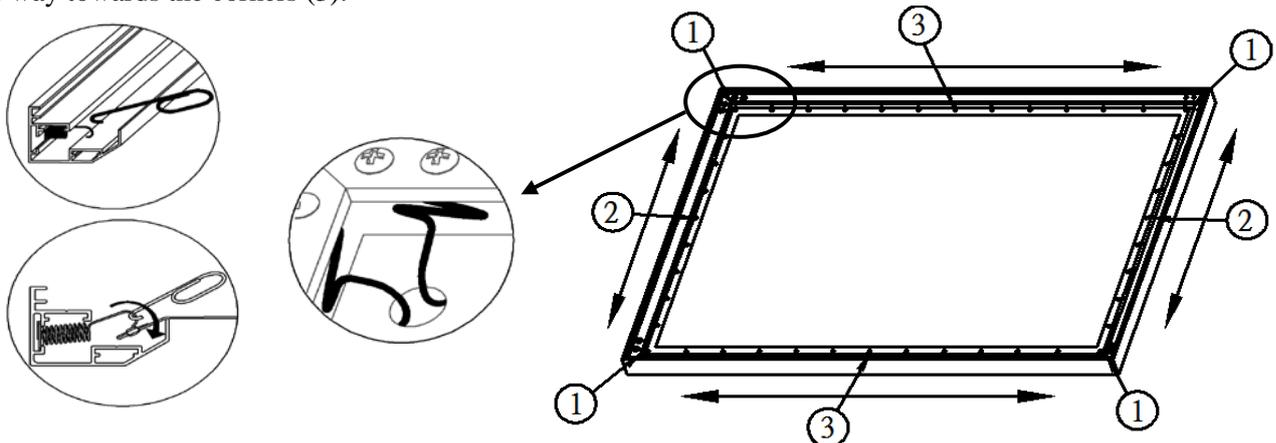
**Step 9.** Insert the Center Support Bar into the upper top groove on the back of the frame (not the one where the spring inserts) with the bottom end near the approximate center point of the frame. Rotate it in at an angle so that both ends of the bar are in alignment with the groove. (See illustrations below for details)
